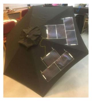
Ebbah Sustainovation approached CPE to seek optical expertise to develop a product for the lighting and ventilation of tents / parasols powered by solar panels.
